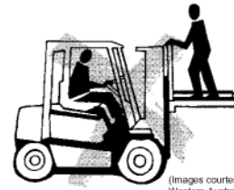
Never raise or carry a person on the tynes of a forklift.
