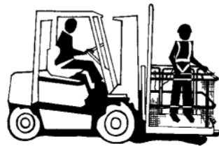
A forklift platform with the user wearing a safety harness and lanyard.
